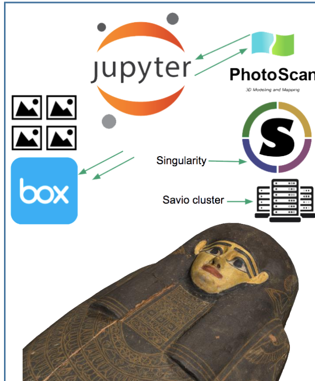
Photogrammetry workflow using Jupyter notebook, Box for data storage/transfer, and Photoscan software in a Singularity container. Example 3D model of ancient Egyptian sarcophagus from Prof. Rita Lucarelli.
