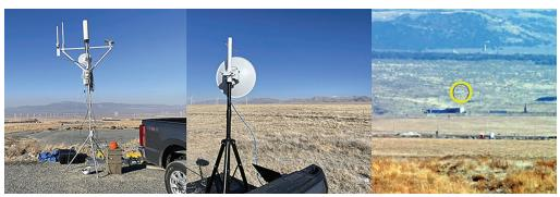
(Pictured from left): The test tower set up on a sensor pad in Fervo, Utah; the Wi-Fi HaLow unit at the site's westernmost pad; and a 30x magnified view of the test tower from the HaLow unit's location.
