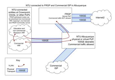
**Figure 1:** NTU Aggregation Point Design BiSON-West is still in the planning stage and the team is working to secure funding and formalize support for the aggregation point. This effort does not fit cleanly in a traditional NSF CC\* grant, so we are exploring state, federal, and private funding opportunities.
